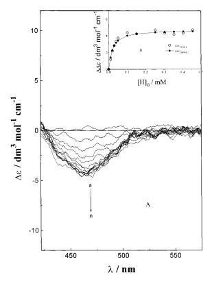
Figure 4. (A) ICD spectral changes of phosphate buffer solution of Methyl Orange (10.7  $\mu$ M) in the presence of 6,6'-(*o*-phenylenediseleno)-bridged bis( $\beta$ -cyclodextrin) **2**. The concentration of host **2** (from a to n): 0, 10, 20, 30, 40, 50.6, 101.1, 151.7, 202.2, 252.8, 303.4, 353.9, 404.4, and 455  $\mu$ M, respectively. (B) Least-squares curve-fitting analysis for the complexations of Methyl Orange with 2.
